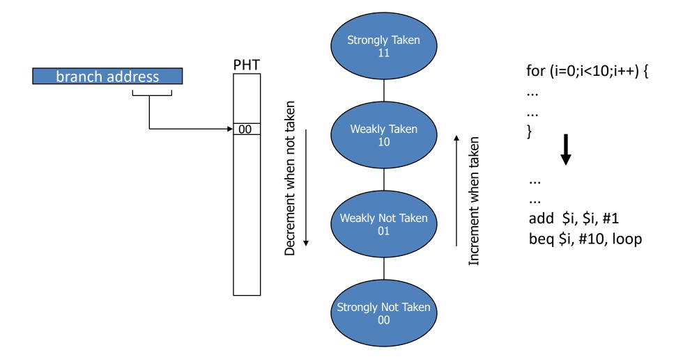
Suppose we have the following branch pattern. What is the accuracy of a 1-bit and 2-bit branch predictors. Assume initial values of 1 (1-bit) and (10) 2-bit.
